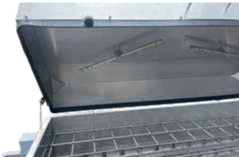
Spinning washer wands clean and sanitize the outside during the bottle wash cycle.
