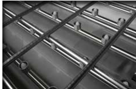
Easy loading grid features cone spray nozzles for clean spray and excellent bottle coverage.
